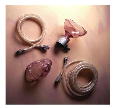
The Air Break Breathing Assembly is designed to provide medical breathing air to a patient with minimal respiratory support. The Demand Valve works on a regulated gas supply 70 to 90 p.s.i.g. and reduces this pressure to a physiologically acceptable level on demand. The Air Break Breathing Assembly includes the demand valve, hoses and fittings pass thru assembly and two adult masks.
